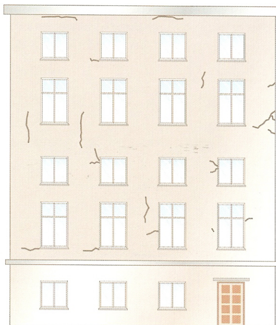
Diffused fractures on the facade
